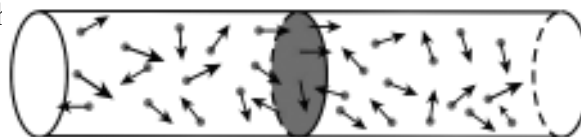
Random motion of electrons (in open circuit)
